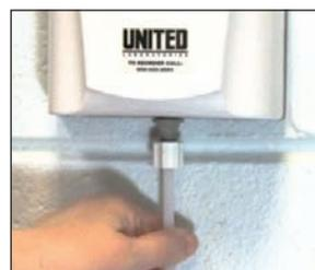
1. Slide the flat, back side of the plastic nut and sleeve assembly over the tubing so it will face down toward the drain.
